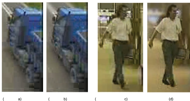
Figure 8. Details of sequences encoded at 150 kbit/s: (a) Frame 44 of Highway MPEG-1 encoded; (b) Frame 44 of Highway MPEG-1 encoded after perceptual pre-filtering (c) Frame 280 of Hall Monitor MPEG-1 encoded; (d) Frame 280 of Hall Monitor MPEG-1 encoded after perceptual pre-filtering; notice that the front left wheel of the truck is visible with semantic pre-filtering only (b). The person's facial features and clothes are clearly visible in (d), whereas they are corrupted by coding artifacts in (c).
