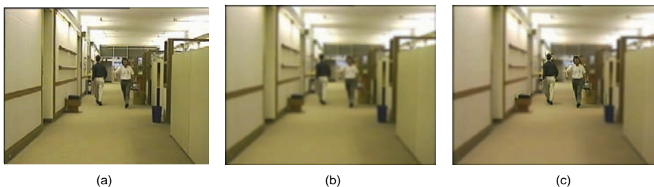
Figure 6. Simplification of contextual information: (a) Sample frame from the test sequence Hall Monitor; (b) simplification of the whole frame using a low-pass filter; (c) selective low-pass filtering based on semantic segmentation results allows one to simplify the information in the background while still retaining essential contextual information
