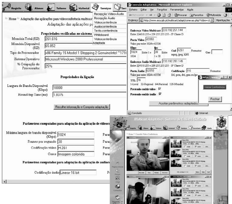
Figure 3. E-learning system screenshots and MMC's adaptation HTML forms based on available QoS
