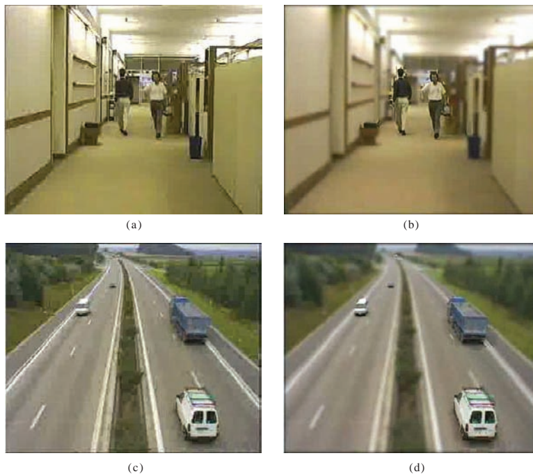
Figure 7. Comparison between standard MPEG-1 encoding and perceptually pre-filtered MPEG-1 encoding at 150 kbit/s. Frame 190 of Hall Monitor: (a) MPEG-1 encoded; (b) MPEG-1 encoded after perceptual pre-filtering; Frame 44 of Highway (c) MPEG-1 encoded; (d) MPEG-1 encoded after perceptual pre-filtering. It is possible to notice that coding artifacts are less disturbing on objects of interest in (b) and (d) than in (a) and (c), respectively.
